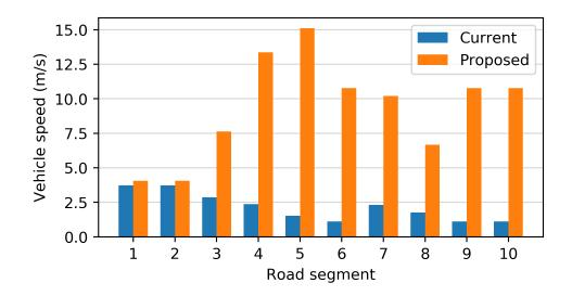
FIGURE 4.3: Comparison of segments speed in sector C
