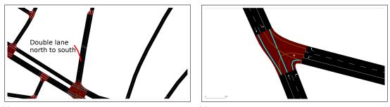
(a) Solution for sector A: double lane for direct right (b) Solution sector B: traffic light in junction allowing turn right turns in red
