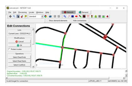
FIGURE 2.1: NETEDIT window: interface to modify the network file, traffic demand and additional elements.
