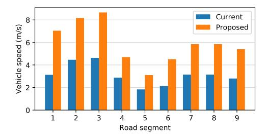
FIGURE 4.5: Comparison of segments speed in sector E
