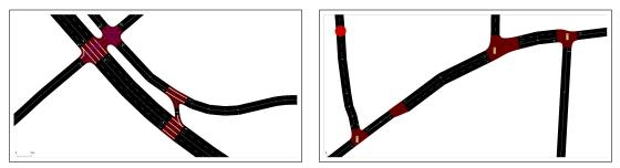
(c) Solution sector C: early entrance in the way from (d) Solution sector D: adjusted timing in 3 traffic lights east to north
