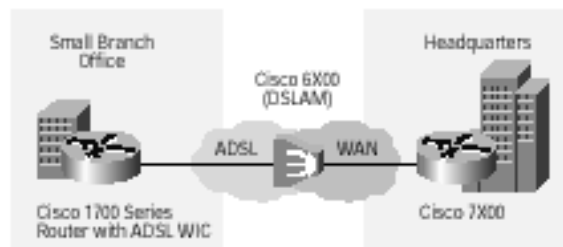
Figure 2 The Cisco 1700 Series Deployed with an ADSL WIC
