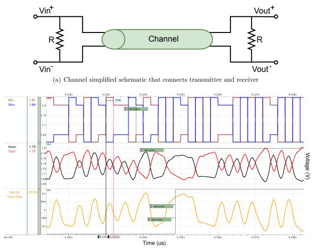
(b) Channel simulation results of 2 meter length at 5 Gbps
