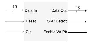
Figure 4.2: Block diagram of the Input Detect Unit of the Elastic Buffer for USB 3.0
