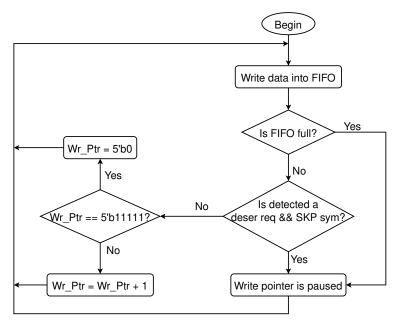
(c) Flow diagram for the desertion operation
