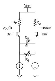
Figure 3.12: CTLE circuit representation. Adapted from [45]
