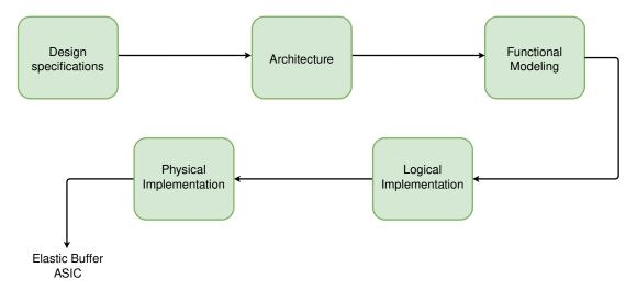
Figure 1.1: Simplified process steps for the design of a digital IC block using a top-down approach
