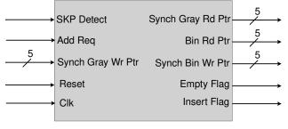
(a) Top block diagram of Read Pointer Generator
