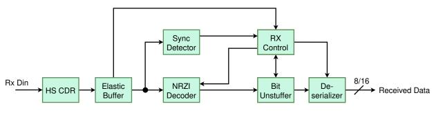
Figure 3.26: USB 2.0 receiver simplified block diagram
