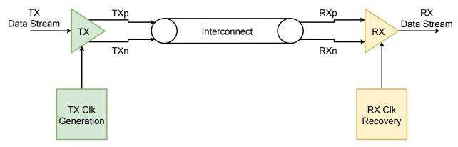
(a) Simplified diagram of the simulation setup for a single differential lane
