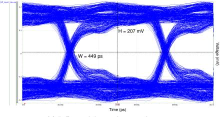
The first analysis is with a data rate of 1 Gbps and a cable length of 1 meter. This description involves two analyses and these are the differential data with and without equalization
