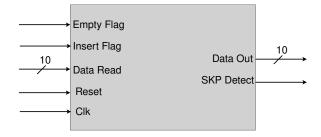
Figure 4.8: Block diagram of the Output Detect Unit of the Elastic Buffer for USB 3.0
