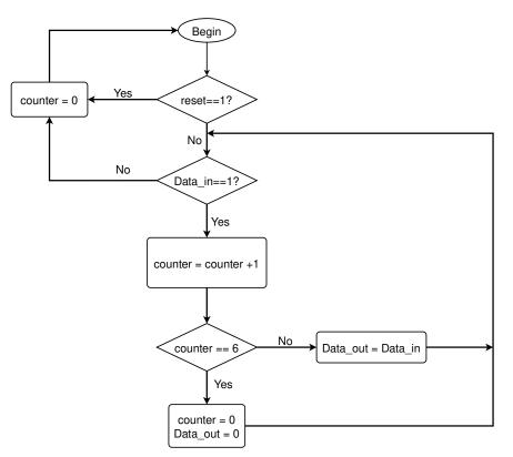
(a) Bit stuffer flow diagram. Adapted from [51]
