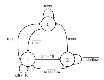
Figure 4.15: FSM state diagram for reading operation for USB 2.0
