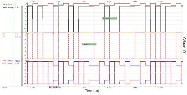
(b) Feed-forward equalizer simulation results at 5 Gbps
