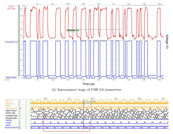
(c) Receiver stage of USB 2.0 transceiver
