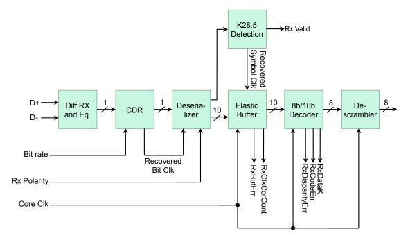
Figure 3.10: USB 3.0 receiver simplified block diagram
