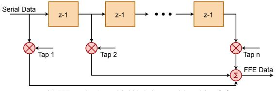
(a) FFE equalizer's simplified block diagram. Adapted from [38]
