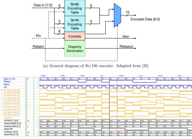
(b) 8b/10b encoder simulation results at 500 MHz
