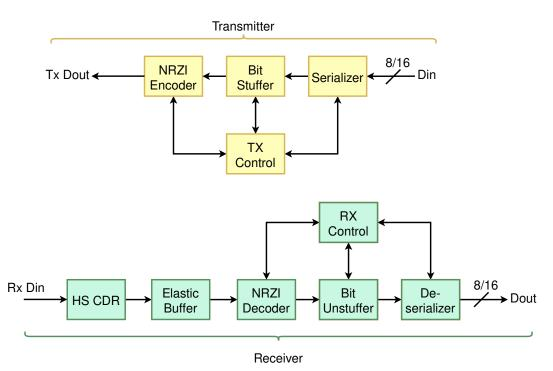
(b) Simplified block diagram of a serial transceiver for USB 2.0 standard. Adapted from [9]
