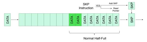
Figure 2.7: EB block diagram for a USB 3.0 implementation. Adapted from [21]
