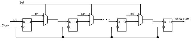
(a) Serializer's simplified schematic. Adapted from [37]
