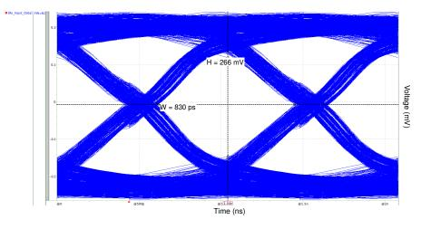
Figure 5.11: Eye-Diagram comparison at the input receiver stage 480 Mbps and 1 meter of length with error insertion
