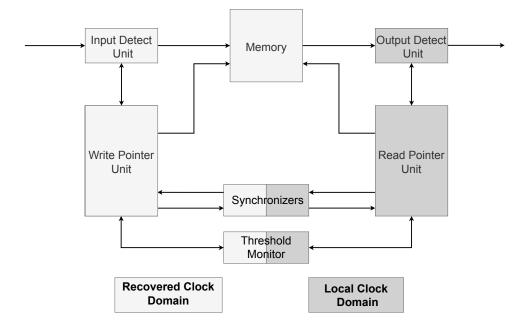
Figure 4.1: Simplified block diagram of Elastic Buffer for USB 3.0
