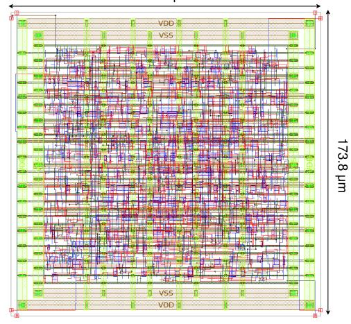
Figure 4.21: Layout of the Elastic Buffer for the USB 2.0 standard
