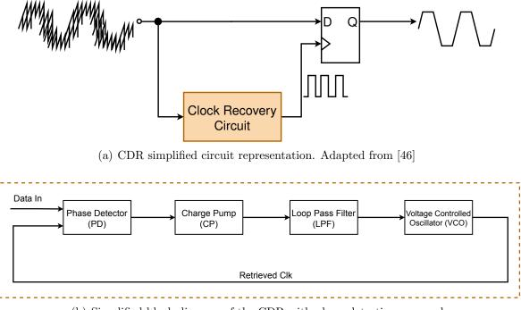
(b) Simplified block diagram of the CDR with phase detection approach
