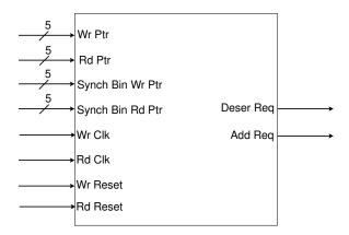
Figure 4.5: Block diagram of the Threshold Monitor Unit of the Elastic Buffer for USB 3.0
