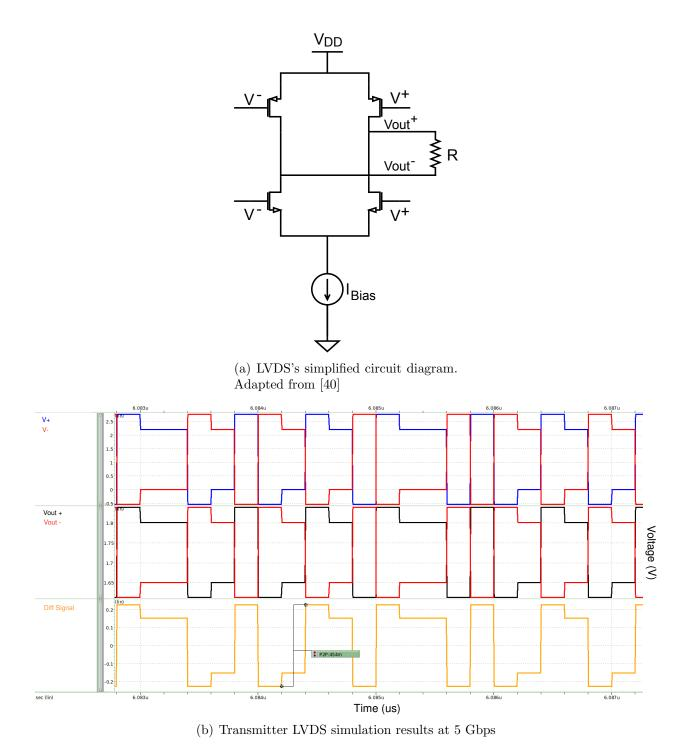
Figure 3.8: LVDS circuit description and event-driven simulation of its behavioral AMS model
