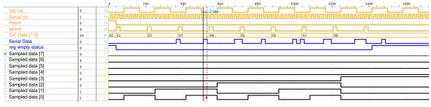
(b) Serializer simulation results at 480 MHz
