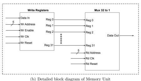
Figure 4.13: Memory Unit of the Elastic Buffer for USB 2.0
