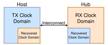
Figure 3.16: Clock domains representation of USB transceiver
