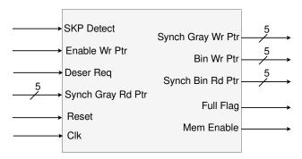
(a) Top block diagram of Write Pointer Generator
