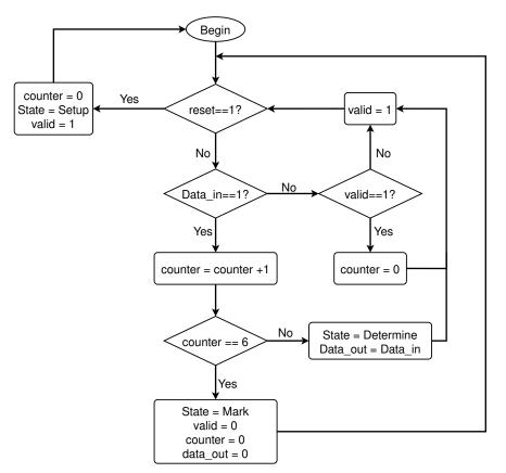
(a) Bit unstuffer flow diagram. Adapted from [51]
