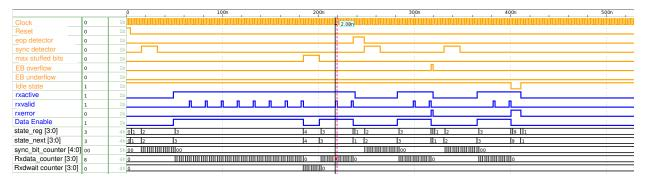
(b) Receiver control FSM simulation results at 480 MHz
