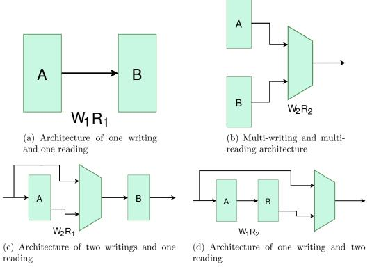
Figure 2.3: Elastic buffer data flow architectures. Adapted from [14]
