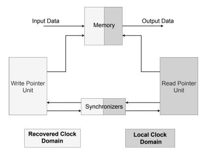
Figure 4.10: Simplified block diagram of Elastic Buffer for USB 2.0
