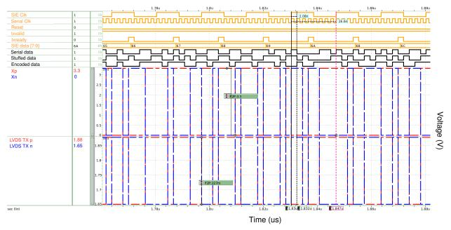
(a) Transmitter stage of USB 2.0 transceiver
