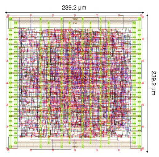
Figure 4.18: Layout of the Elastic Buffer for the USB 3.0 standard
