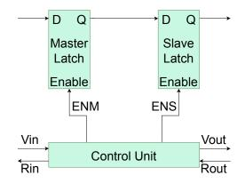
Figure 2.5: Topology of the EB master-slave flip-flop. Adapted from [19]
