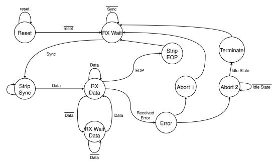
(a) State diagram of the receiver FSM. Adapted from [49]
