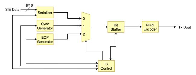
Figure 3.19: USB 2.0 transmitter simplified block diagram
