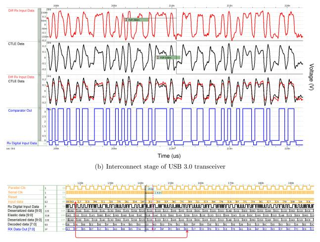
(c) Receiver stage of USB 3.0 transceiver
