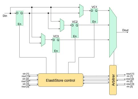
Figure 2.6: Elastistore architecture. Adapted from [18]
