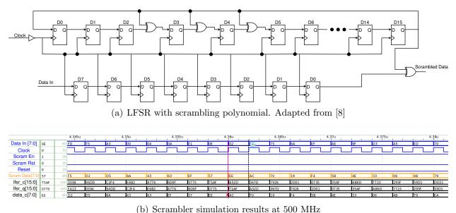
Figure 3.3: Scrambler block diagram description event-driven simulation of its behavioral AMS model
