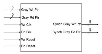
(a) Simplified block diagram of Synchronizers
