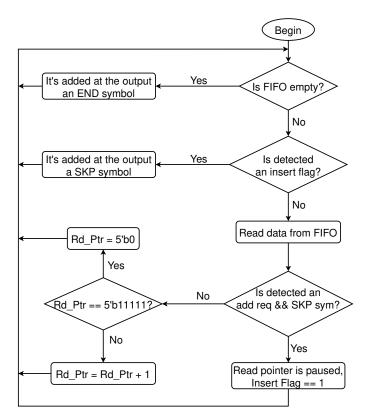
Figure 4.9: Flow diagram for the addition operation
