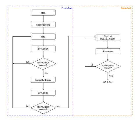
Figure 4.16: Flow diagram for a digital flow synthesis
