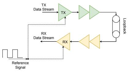
(b) Loopback configuration used for USB transceiver simulations
