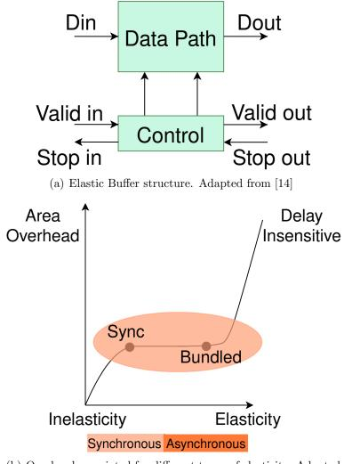
(b) Overhead associated for different types of elasticity. Adapted from [16]
