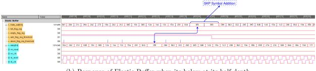
(b) Response of Elastic Buffer when its below at its half depth
