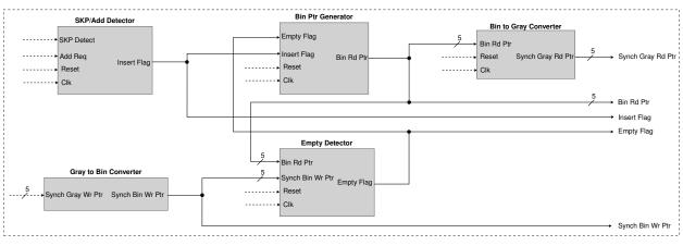
(b) Detailed block diagram of Read Pointer Generator
