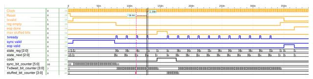
(b) Transmitter control FSM simulation results at 480 MHz
