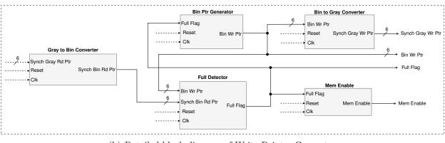
(b) Detailed block diagram of Write Pointer Generator
