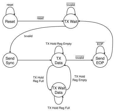
(a) State diagram of the transmitter FSM. Adapted from [49]
