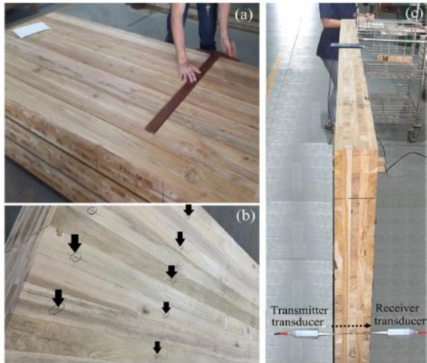
Fig. 2 a CLT panels of Gmelina arborea lumber, b CLT panels of Tectona grandis and c position of the transducer during ultrasound measurement
