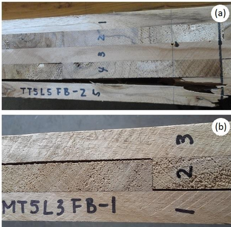
Fig. 3. Failures in flexure test: tension (a) and delamination (b) for the 3- and 5-layer CLT panels of the two species.
