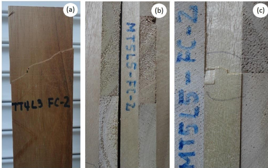
Fig. 5. Failures in compression parallel to the grain test: shearing (a), splitting (b) and crushing (c) for the 3- and 5-layer CLT panels of the two species.
