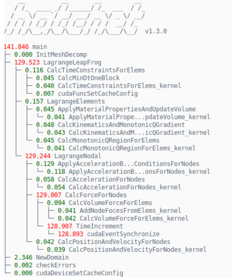
(a) LULESH Call Path Tree created from NSight Systems NVTX trace data
