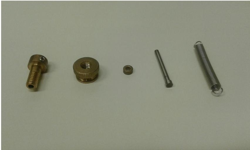
Figure D.2 Spring attachment components: (from left to right) upper bronze coupling, lower bronze coupling, mechanical spacer, stainless steel pin, spring.
