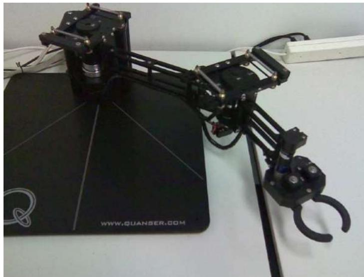
Figure 3.2 2DoF Quanser manipulator physical plant
