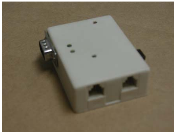
Figura 6.32 Interfaz RS-232/ One Wire.
