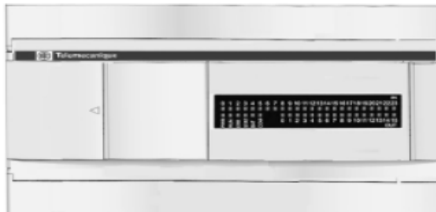
Figura 5.2.1.1 PLC Twido TWDLCE40DRF.
