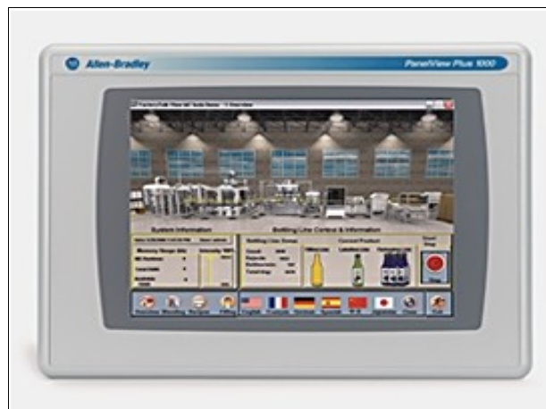
Figura 5.2.8 Pantalla de operador PanelView Plus 1000. [4]
