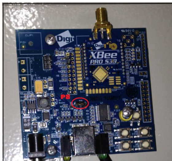
Figura 5.2 Jumper de loop-back de tarjeta XBIB-U-DEV
