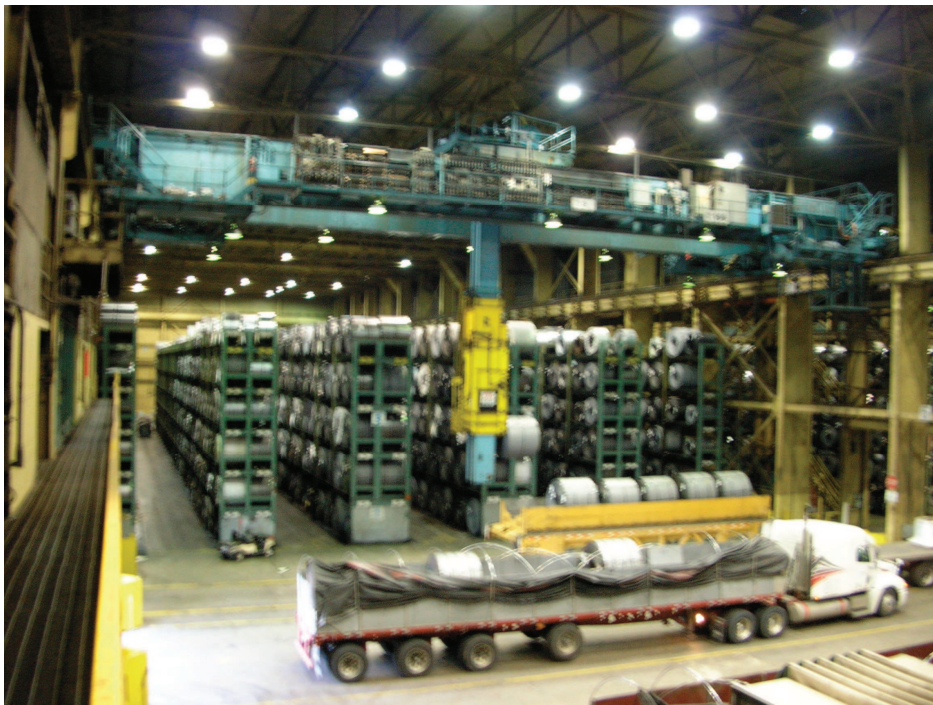
Photo 4 – 25 ton Stacker Crane
