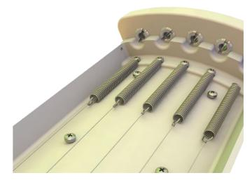
Figure 4-32. Attachment of the springs and muscles.
