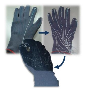
Figure 6-2. Assembly of the Tendon Layout of the Glove
