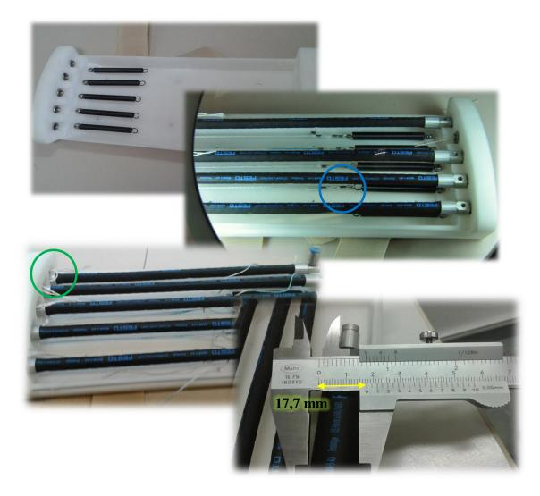
Figure 6-5. Mechanical Support of the Actuators
