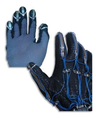
Figure 6-4. Electronic Layer of the Glove
