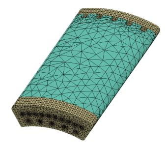
Figure 4-38. Mesh of the support structure of the actuators.
