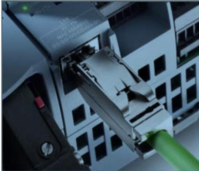
**Figura 4.20. Puerto Ethernet del PLC S7-1200.**
