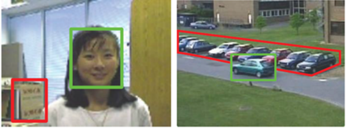
Figure 1.5 Example of clutter: objects in the background red boxes can distract the system because are similar to the target. Left: similar color. Right: similar shape. Taken from [Com01]
