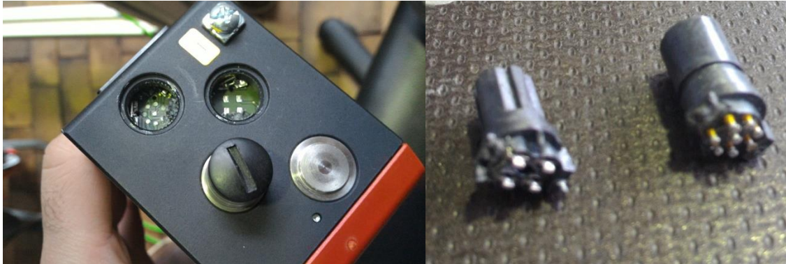
Figure 60 Damage to LPS's connectors
