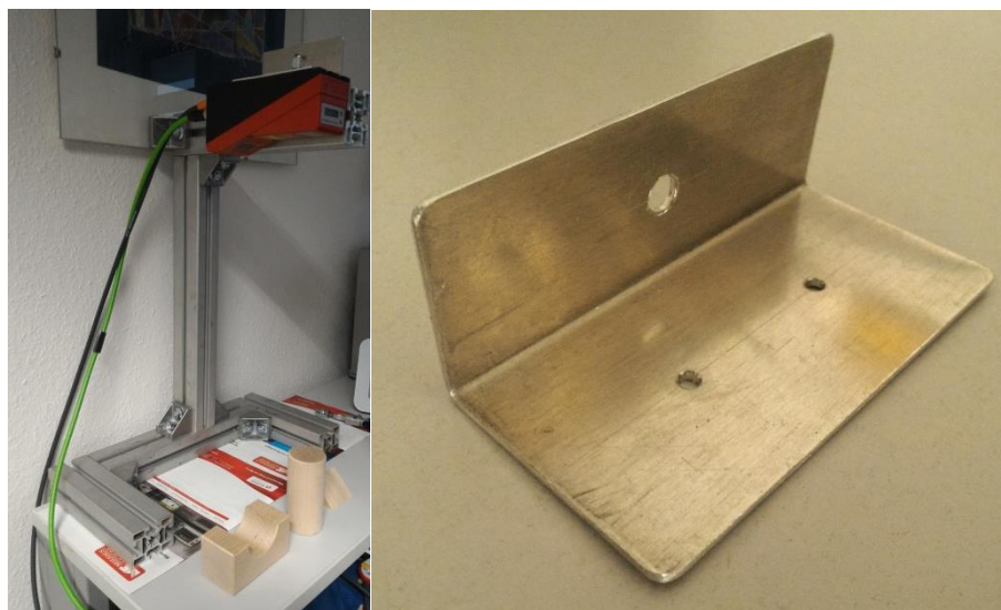
Figure 23 Temporal mounting base for LPS
