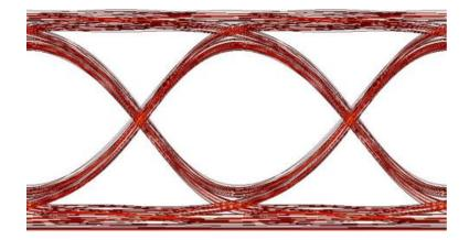
Figure 4.7 SPITDS eye diagram of example A (section 4.1.1) at 10 Gb/s with 256 bits.
