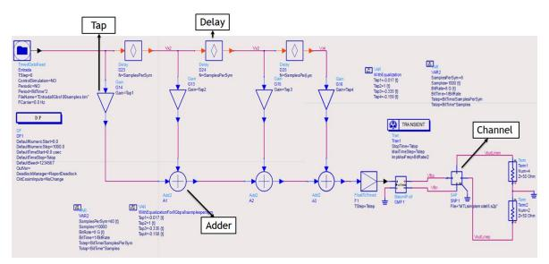
Figure A.3.2 Diagram of the implementation for FFE equalizer in ADS for a differential channel using a s-parameters block.
