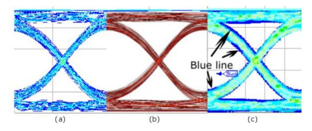
Figure 4.8 Comparison of eyes diagrams from Eye Probe plotter (a), SPITDS (b) and Eye Diagram FrontPanel plotter (c) of example A (section 4.1.1) at 10 Gb/s with 256 bits. The vertical and horizontal scales are 20 ps per division and 0.1 V per division respectively.
