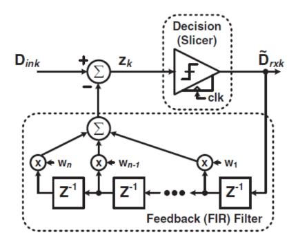
Figure 2.7 Common implementation of a receiver DFE.
