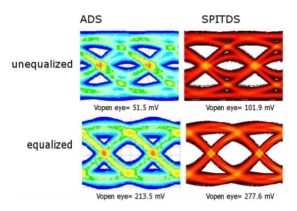
Figure 4.18 Eye diagrams comparison between SPITDS and ADS simulations for a link of example A (section 4.1.1) at 20 Gb/s with 10000 bits. The horizontal scale for all figures is 10 ps per division but the vertical scale is 0.2 V for the unequalized signal and 0.1 for equalized signal diagrams.
