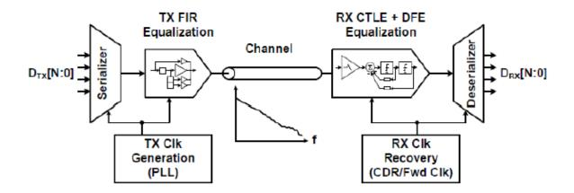
Figure 2.5 High speed serial link with TX FFE equalization and RX CTLE and DFE equalization taken from [13].
