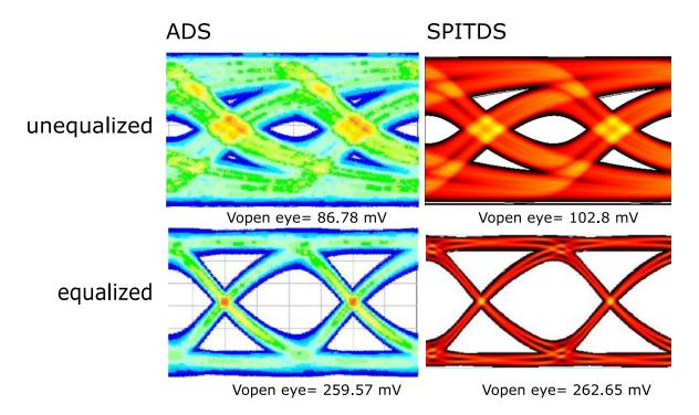
Figure 4.12 Eye diagram comparison of ADS and SPITDS simulations for ADS transmission line model (section 3.2) with equalization at 5 Gb/s with 10000 bits. The vertical and horizontal scales are 50 ps per division and 0.1 V per division respectively.
