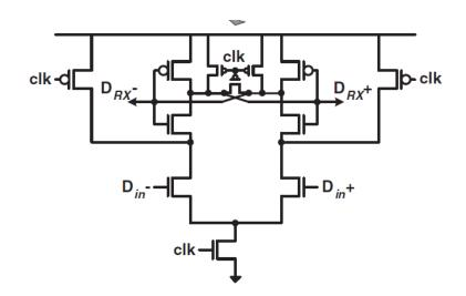
Figure 2.3 Typical receiver input stage with regenerative latch taken from [12].
