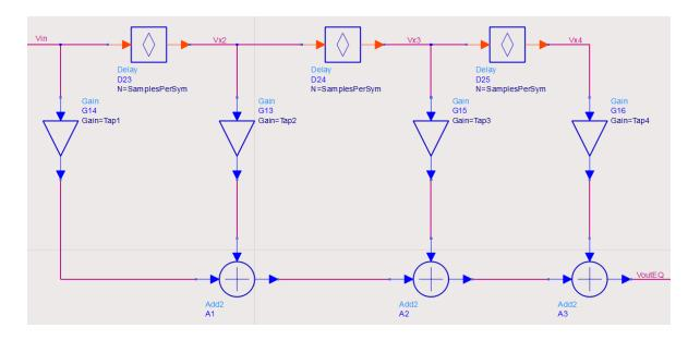
Figure A.3.1 Detail diagram of the implementation for FFE equalizer in ADS.
