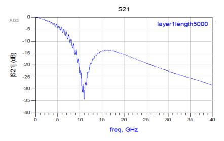
Figure 4.4 Transmission parameters for semianlytical link with stub effect.
