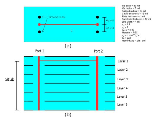
Figure 4.3 Diagram of a link model in MLSS and its main parameters. (a) top view, (b) crosssection. The materials are chosen as a perfect electric conductor and FR4 with the given specifications.
