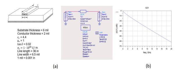
Figure 3.5 ADS transmission line model. (a) Diagram of single ended microstrip line. (b) Transmission parameters of microstrip line.
