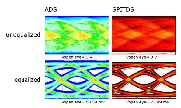
Figure 4.14 Eye diagram comparison of ADS and SPITDS simulations for ADS transmission line model (section 3.2) at 9 Gb/s with 10000 bits. The vertical and horizontal scales are 20 ps per division and 0.1 V per division respectively.
