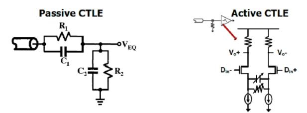
Figure 2.6 Receiver CLTE equalization taken from [13]. (a) passive. (b) active.
