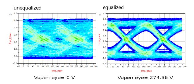
Figure 3.11 Eye diagram comparison for ADS transmission line model at 7 Gb/s with and without equalization using LMS algorithm ADS implementation with a differential channel with 36 inches long.
