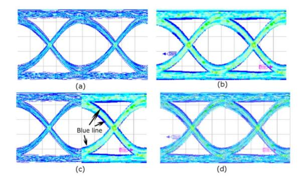
Figure 4.6 Eye diagram of example A (section 4.1.1) at 10 Gb/s with 256 bits. The vertical and horizontal scales are 20 ps per division and 0.1 V per division respectively. (a) eye diagram from Eye Probe plotter. (b) eye diagram from Eye Diagram FrontPanel plotter. (c) comparison between these two plotters. (d) both eye diagrams superposed.
