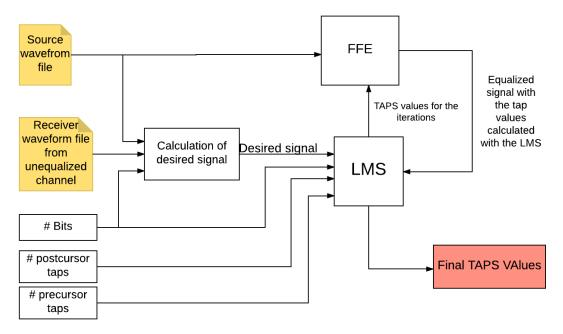
Figure 3.13 Diagram for the implementation of a LSM algorithm adaptation for a FFE.
