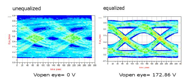
Figure 3.7 Eye diagram comparison for ADS transmission line model at 7 Gb/s with and without equalization using LMS algorithm ADS implementation with a single ended channel model with 36 inches long.
