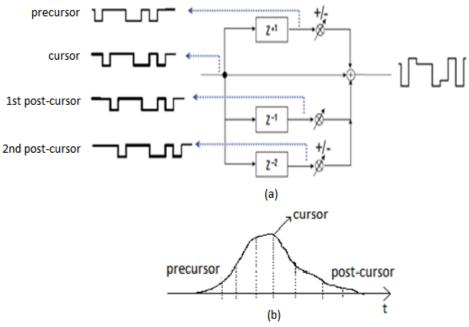
Figure 2.9 Predistortion of the signal by 4 taps FFE taken from [14] (a). Impulse response equalization effect (b).
