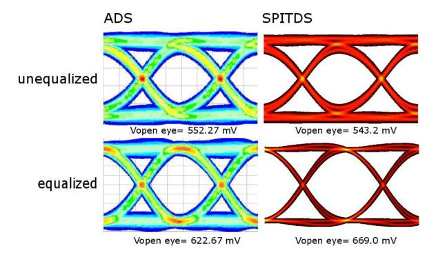
Figure 4.16 Eye diagrams comparison between SPITDS and ADS simulations for a link of example A (section 4.1.1) at 10 Gb/s with 10000 bits. The horizontal scale for all figures is 20 ps per division, the vertical scale is 0.2 V for the unequalized signal and 0.1 V for equalized signal diagrams.
