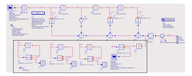
Figure 3.3 Diagram of FFE with LMS algorithm ADS implementation.
