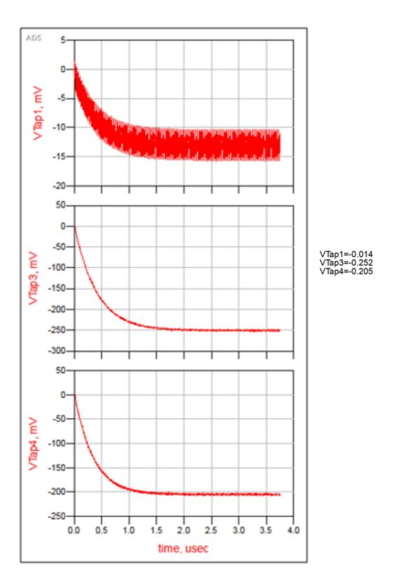
Figure 3.6 Convergence of the LMS algorithm ADS single ended channel implementation.
