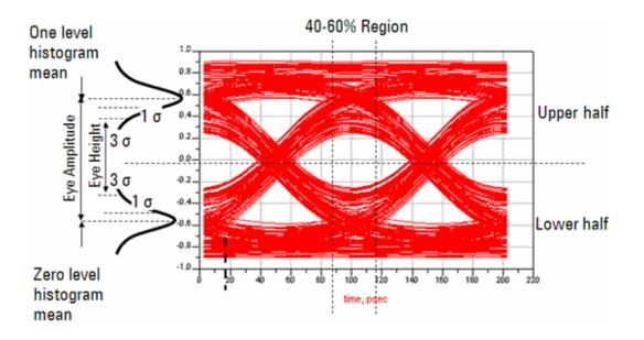
Figure 4.9 ADS eye height measurements, taken from [19].
