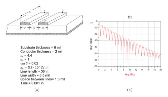
Figure 3.9 ADS transmission line model. (a) Diagram of microstrip coupled lines. (b) Transmission parameters of microstrip line.
