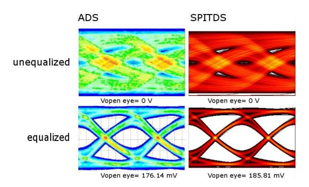
Figure 4.13 Eye diagram comparison of ADS and SPITDS simulations for ADS transmission line model (section 3.2) at 7 Gb/s with 10000 bits. The vertical and horizontal scales are 20 ps per division and 0.1 V per division respectively.
