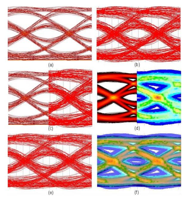
Figure A.4.2 Comparison between SPITDS and ADS eye diagrams for a link of example B (section 4.1.1) at 15 Gb/s without equalization. (a) Eye diagram from SPITDS with 256 bits. (b) eye diagram from ADS with 256 bits. (c) comparison of ADS and SPITDS with a 256 bits. (d) comparison of ADS and SPITDS with 10000 bits. (e) eye diagram from ADS and SPITDS with 256 bits eye superposed. (f) eye diagram from ADS and SPITDS with 10000 bits eye superposed.
