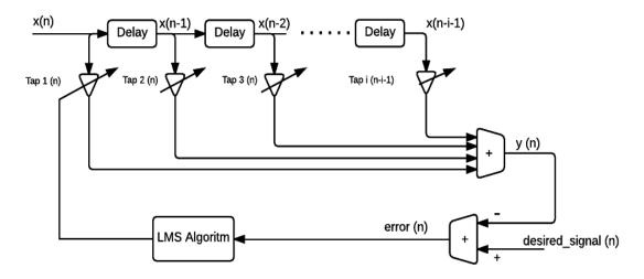
Figure 3.14 Detail of the LMS algorithm equalizer process (FFE) and adaptive taps process (LMS algorithm).
