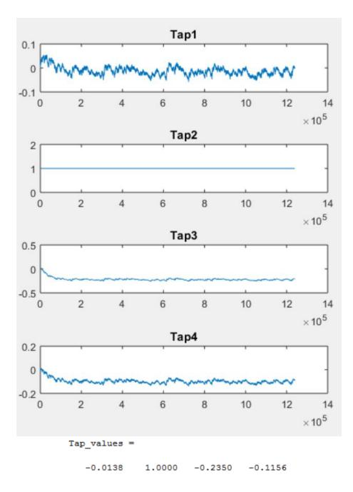
Figure 3.15 Convergence of the LMS algorithm and taps values applied at SPITDS data.
