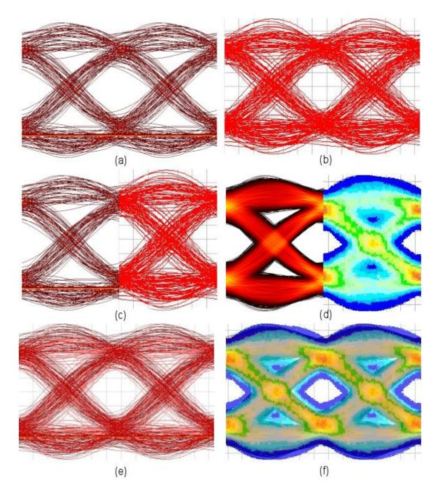
Figure A.4.3 Comparison between SPITDS and ADS eye diagrams for a link of example B (section 4.1.1) at 15 Gb/s with equalization. (a) Eye diagram from SPITDS with 256 bits. (b) eye diagram from ADS with 256 bits. (c) comparison of ADS and SPITDS with a 256 bits. (d) comparison of ADS and SPITDS with 10000 bits. (e) eye diagram from ADS and SPITDS with a 256 bits eye superposed. (f) eye diagram from ADS and SPITDS with 10000 bits eye superposed.
