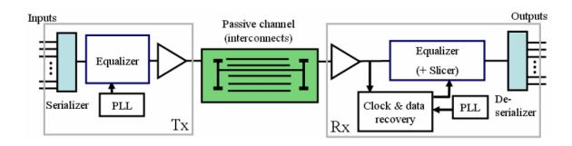
Figure 2.1 Diagram of a high-speed serial link (SerDes) taken from [4].
