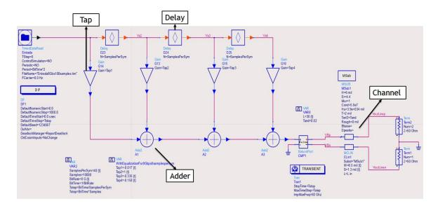
Figure 3.2 Diagram of the implementation for FFE equalizer in ADS for a differential channel.
