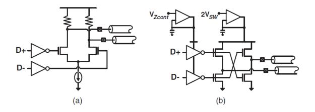
Figure 2.2 Typical transmitter topology. (a) current mode driver. (b) Voltage mode driver taken from [12].
