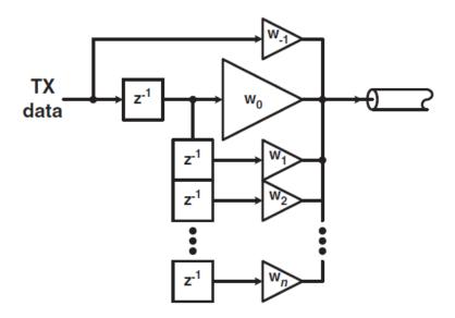
Figure 2.8 Common implementation of a transmitter FFE equalization taken from [12].
