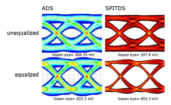
Figure 4.17 Eye diagrams comparison between SPITDS and ADS simulations for a link of example A (section 4.1.1) at 15 Gb/s with 10000 bits. The horizontal scale for all figures is 20 ps per division but the vertical scale is 0.2 V for the unequalized signal and 0.1 V for equalized signal diagrams.
