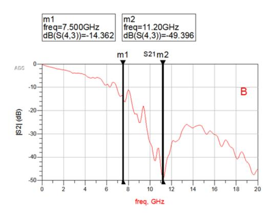
Figure 4.19 Transmission parameters magnitude for thee link of example B (4.1.1) simulations. The two fundamental frequency for 15 and 22.4 Gb/s are shown.
