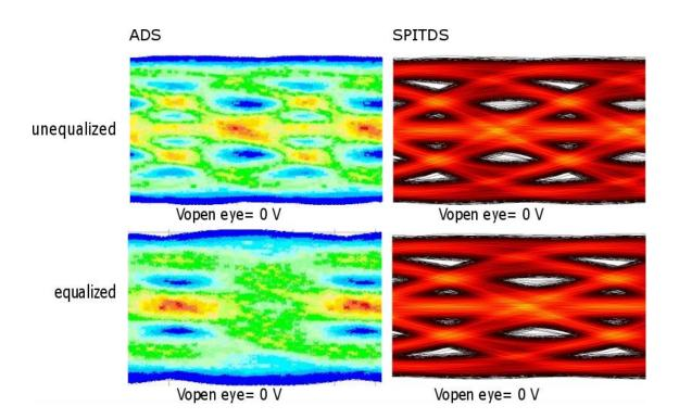
Figure 4.21 Eye diagrams comparison between SPITDS and ADS for a link of example B (section 4.1.1) at 22.4 Gb/s, near of the notch. The vertical and horizontal scales are 10 ps per division and 0.1 V per division respectively.
