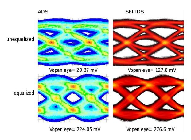
Figure 4.20 Eye diagrams comparison between SPITDS and ADS simulations for a link of example B (section 4.1.1) at 15 Gb/s. The vertical and horizontal scales are 10 ps per division and 0.2 V per division respectively.
