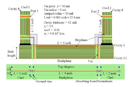
Figure 4.1 Diagram of the link and model parameters taken from [1].
