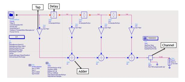
Figure 3.1 Diagram of the implementation for FFE equalizer in ADS with single ended channel.
