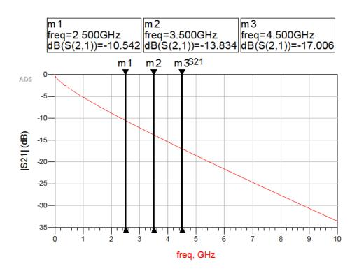
Figure 4.11 Transmission parameter magnitude for the ADS transmission line model (section 3.2) simulations. The three fundamental frequency for 5, 6 and 9 Gb/s are shown.
