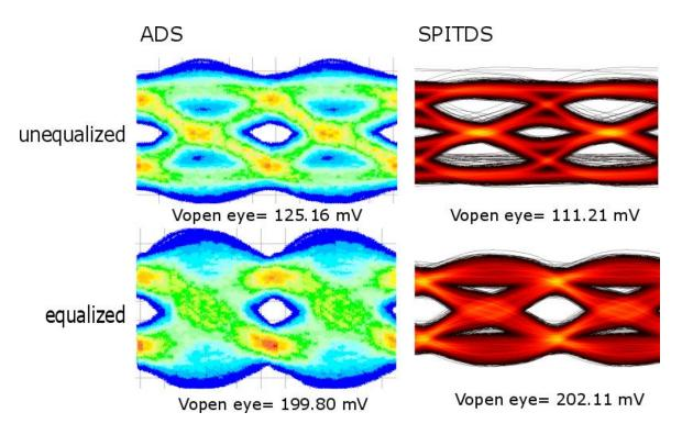
Figure 4.22 Eye diagram comparison for MLSS model with 5000 mil of length (L=5000 mil) for the trace (section 4.1.2) at 18 Gb/s with 1000 bits. The vertical and horizontal scales are 10 ps per division and 0.2 V per division respectively.
