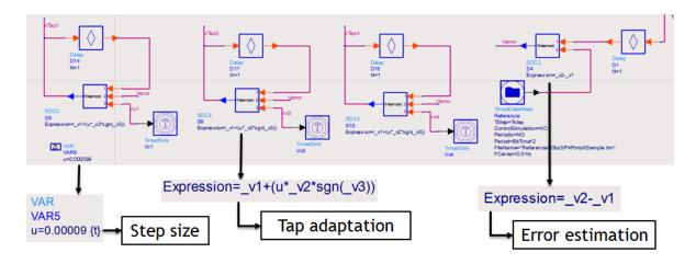
Figure 3.4 Detail view of LMS algorithm implementation in ADS.
