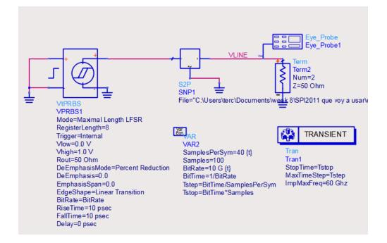
Figure 4.5 Circuit in ADS for eye diagrams from Eye Probe and Eye Diagram FrontPanel plotters comparisons.
