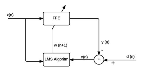
Figure 2.10 Block diagram of LMS algorithm applied at an adaptive FFE.
