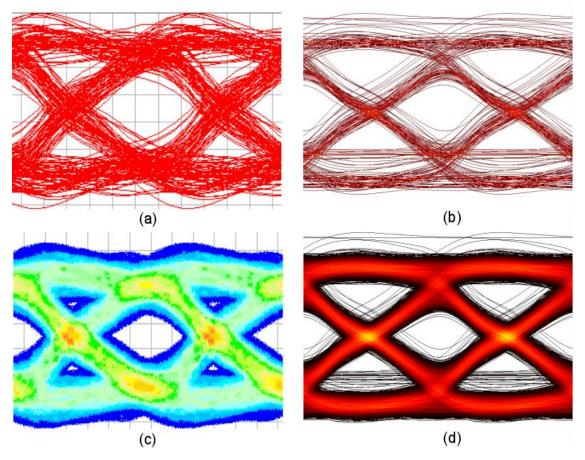
Figure 4.23 Comparison between SPITDS and ADS eye diagrams for a link of example section 4.1.2 at 15 Gb/s without equalization. (a) eye diagram from ADS with 256 bits. (b) eye diagram from SPITDS with 256 bits. (c) eye diagram from ADS with 10000 bits. (b) eye diagram from SPITDS with 10000 bits. (c). The vertical and horizontal scales are 10 ps per division and 0.2 V per division respectively
