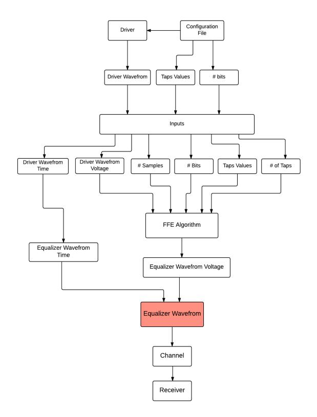
Figure 3.12 Diagram of the implementation for FFE equalizer in SPITDS.
