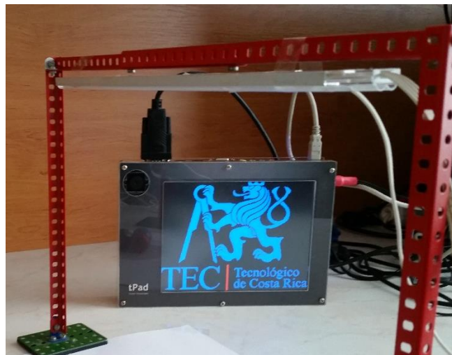
Figure 7.2. Illumination structure for the scene and welcome screen for the Computer Vision System.
