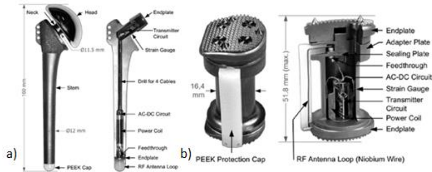
Figure 2.2.3. Instrumented shoulder endoprosthesis and section view to depict the sensing electronics (a) and Instrumented vertebral body and section model to depict electro-mechanical measurement system (b). Adapted from [57]
