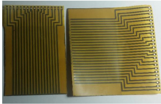
Figure 4.1.2. Actual printed vertical and horizontal electrodes on the polyamide substrate (with adhesive layer on).
