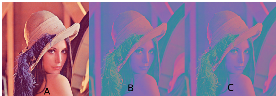
Figure 6.2: Color space transformation in the Beagleboard XM. A) Base image. B) Octave representation of algorithm. C) Conversion by the GPP 3
