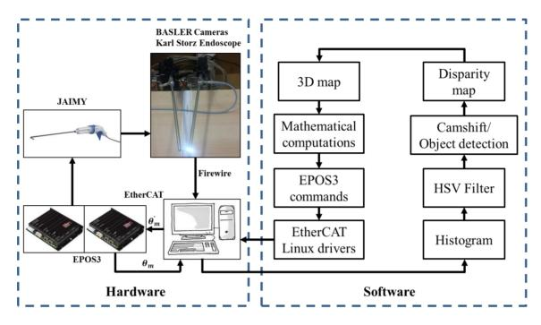
Figure 22. Block diagram of the solution.
