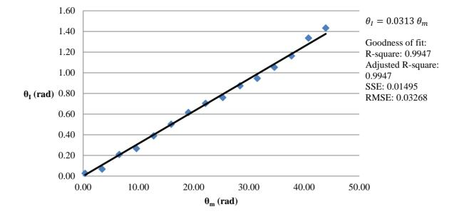
0.078 mm and  $e = 0.0149 (rad)^2$ . The method of linear regression is also used in order to verify the previously estimated value. For this case the Matlab Curve Fitting Tool is used.
