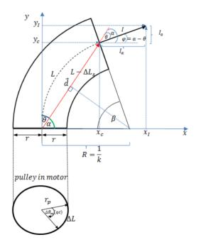
Figure 9. Kinematic model of the JAYMI<sup>TM</sup> instrument.
