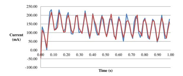
Figure 15. Current controller response after auto tuning, blue  $\rightarrow$  current demand value, red  $\rightarrow$  current actual value.
