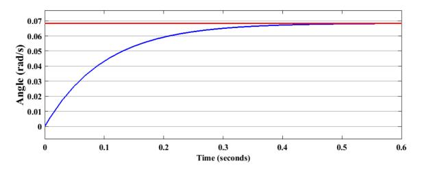
Figure 13. Kinematic model simulation result considering ideal dc motor model.
