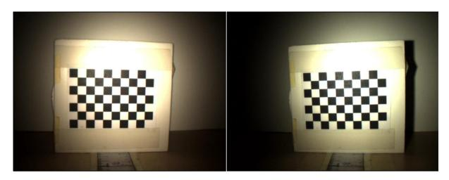
Figure 17. First pair image of the pictures used to do the stereo calibration.
