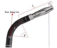
Figure 8. Flexible section of the JAIMY<sup>TM</sup> instrument.
