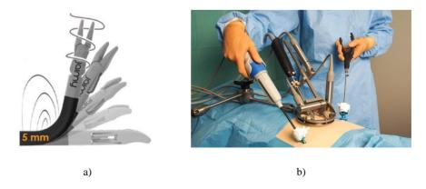
**Figure 6.** a) Bending, tip rotation and grasping are the 3DOF of JAIMY<sup>TM</sup>, b) Laparoscopy surgery application, images taken from [2].
