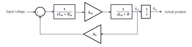
Figure 10. Mathematical model of a commercial DC Motor where  $k_m = k_b$ .
