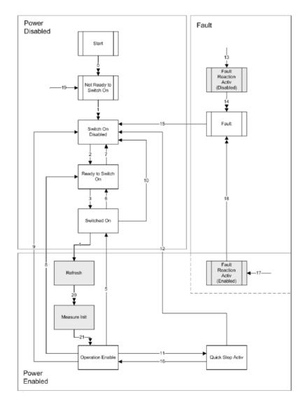
Figure 27. EPOS3 state machine, taken from [25].
