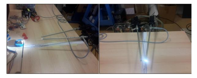
Figure 18. Endoscopic lenses plus Basler cameras setup.
