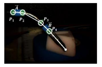
Figure 19. Image of the tip of the JAIMY<sup>TM</sup> being tracked by using markers.
