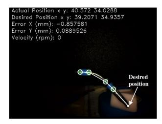
Figure 23. Automatic positioning of the tip of the JAIMY<sup>TM</sup> in the desired point.
