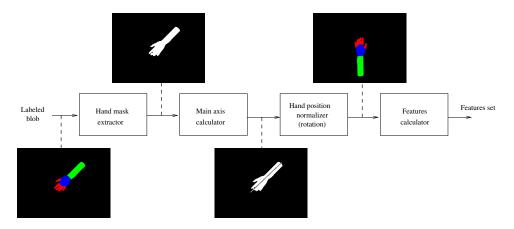
Figure 4.4: Features extraction process for hand pose classification
