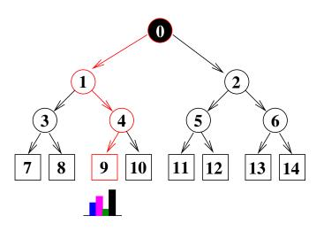
Figure 3.3: Prediction process for a decision tree. The processing path of a data point is marked in red.
