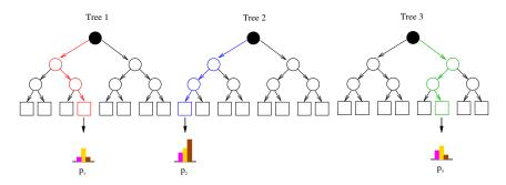
Figure 3.4: Graphical description of random decision forest (T = 3 and depth = 4). The 3 prediction paths are marked in red, blue and green producing 3 corresponding probability distributions.
