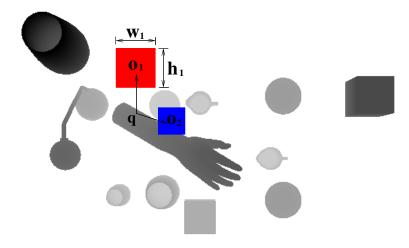
Figure 4.3: Example of Curfil's feature calculation in a depth image
