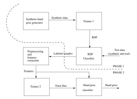
Figure 4.1: General diagram of the system developed
