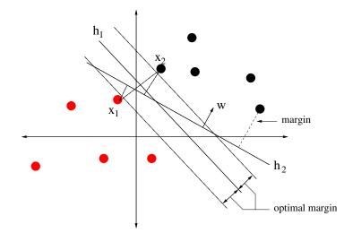
Figure 3.5: Features space separation using hyperplanes.
