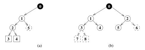
Figure 3.2: Decision tree training algorithms. (a) Depth-first method. (b) Breadth-first method.
