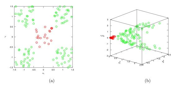
Figure 3.6: Feature space mapping using kernels. a) Original 2D data set not directly separable through an hyperplane. b) Mapped data set using  $\phi(\mathbf{x}) = \mathbf{z} = \{x_i^2, x_j^2, x_i x_j\}$  for  $\mathbf{x} = \{x_i, x_j\}$ .
