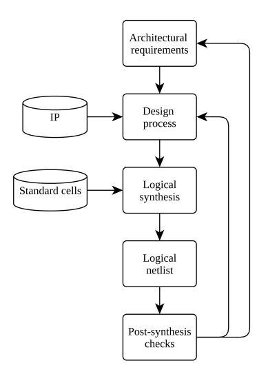
Figure 1.1: ASIC design and synthesis process
