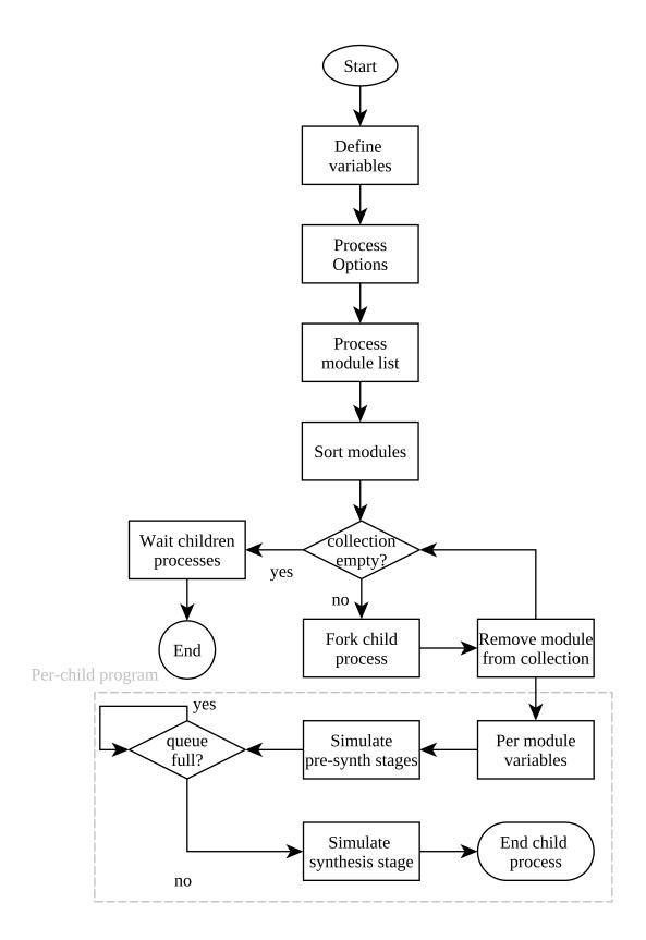
Figure 4.1: Tool execution flow
