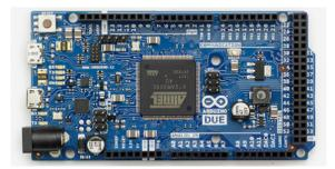
Figure 7.6: Arduino Due board.
