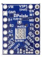
Figure 7.1: Driver for the stepper motors.
