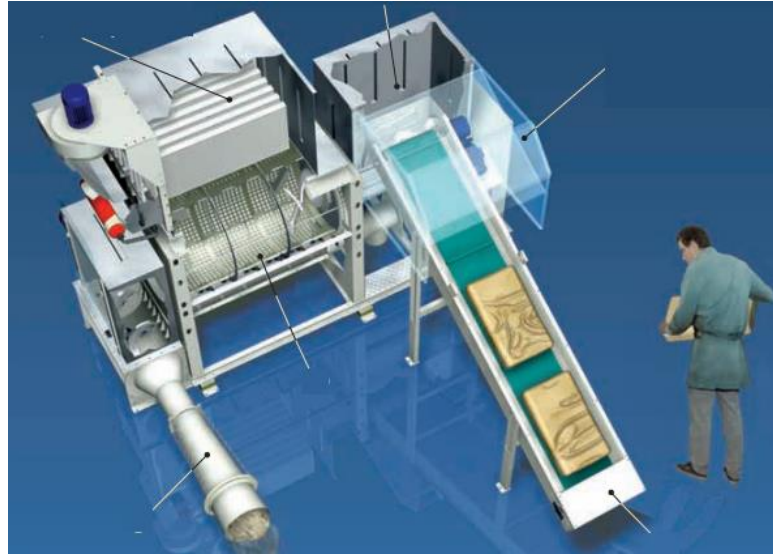
Figura B.3.2. Automatic bag splitter, RSA. Tomado de Wangroup. (2001)
