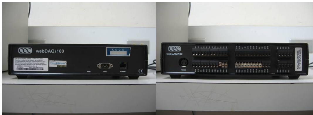
Figura 5.22 Datalogger CEC webDAQ/100 .
